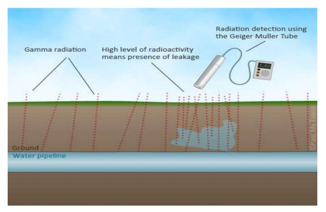
The use of a radioisotope that emits <u>beta</u> radiation is important as beta radiations have the correct <u>penetrating power</u> to travel through the soil to give a measureable reading above ground.
